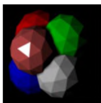
Figure 3: An optical-geometric satellite model represented as six polyhedra partially penetrating each other (a specular flash or glint given off a flat facet can be seen on one of the polyhedra).
