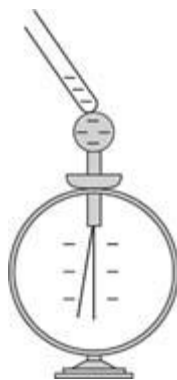
Fig. 1. An electroscope reports the presence of charge.
