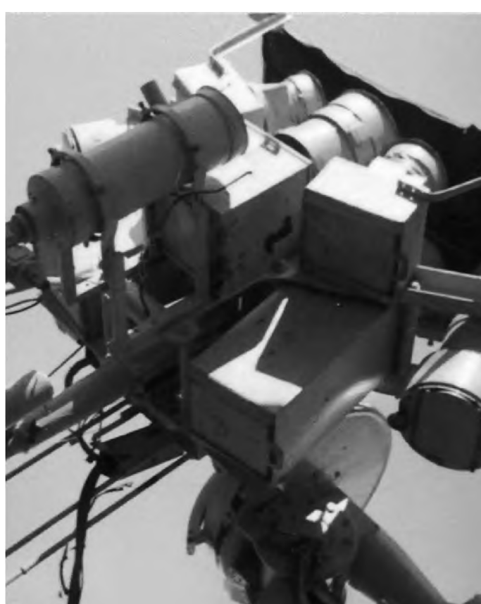
Fig. 3 The 7-camera astrograph was twice modernized. Some cameras were replaced with more efficient ones, their field of view also changed. Thus, all the photographic plates of the astrograph are divided into three series: the Old (1957–1959), the New (1959–1966) and the III (1966–1998) series.
