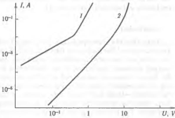
Fig. 1. The VC dependence of the samples: 1 — initial films; 2 — after the electric treatment
