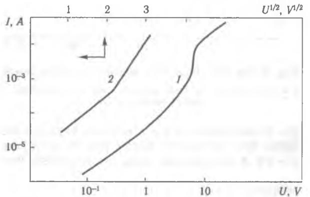
Fig. 2. The VC dependence of the films after annealing in the atmosphere of He
