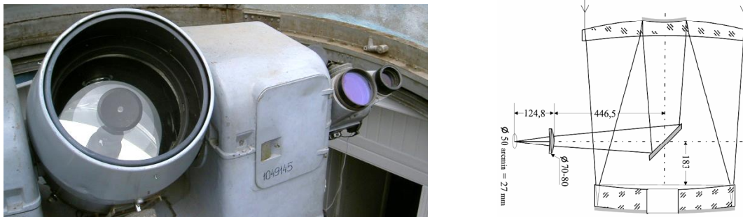
Figure 1: (Right) – Alt-azimuthal KT-50 telescope (photo); (Left) – Optical scheme of telescope.
