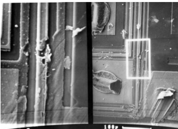
Fig. 1,b. Image of the metallization integrity breaking defect (photolayer etching).
