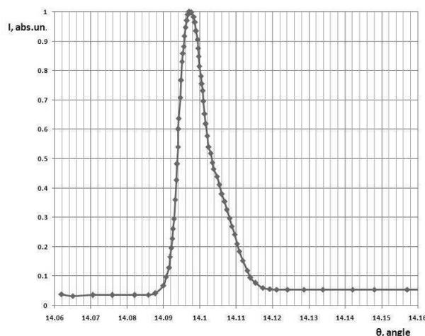
Fig.4 b. The rocking curve (oxide thickness 1.5 micron)
