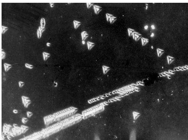
Fig. 3 The electronic image of separate dislocations
