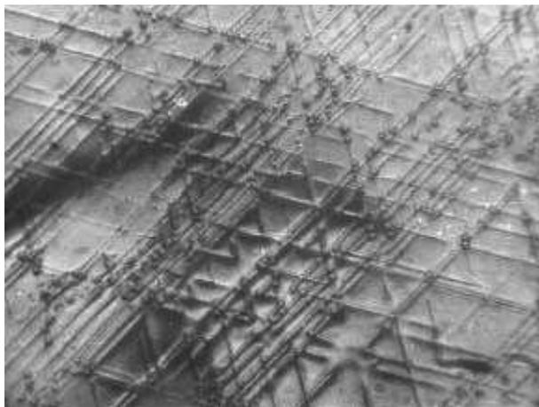
Fig. 2 The electronic image of dislocation networks (1x2300)
