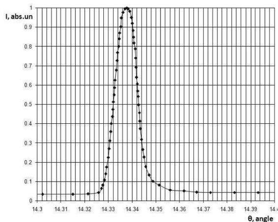
Fig.4 a. The rocking curve (oxide thickness 0.15 micron)
