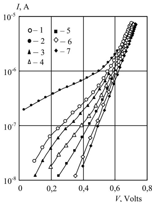
Fig. 1.  $I$ - $V$  characteristics of the forward current of a p-n structure: initial (1) and after S-treatment and subsequent storage in helium: 2 –  $2.4 \cdot 10^3$  s; 3 –  $7.2 \cdot 10^3$  s; 4 –  $1.7 \cdot 10^5$  s; 5 –  $5.2 \cdot 10^5$  s; 6 –  $2.6 \cdot 10^6$  s; 7 –  $7.8 \cdot 10^6$  s
