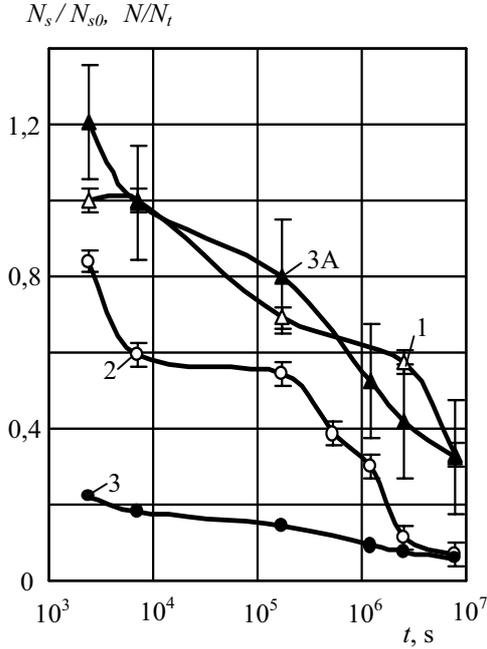
Fig. 4. Effect of the storage duration on the concentrations: 1 –  $N_s/N_s(0)$ ; 2 –  $N/N_i$  in surface non-homogeneities; 3, 3A – average of  $N_s/N_i$  in surface. Ordinate of curve 3A are normalized at  $t=7.2 \cdot 10^3$  s
