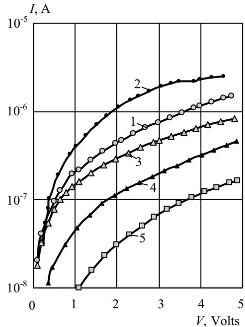
Fig. 3. I–V characteristics of the reverse current of a p–n structure: initial (1) and after S-treatment and subsequent storage in helium: 2 –  $2.4 \cdot 10^3$  s; 3 –  $1.7 \cdot 10^5$  s; 4 –  $1.2 \cdot 10^6$  s; 5 –  $2.6 \cdot 10^6$  s; 6 –  $7.8 \cdot 10^6$  s
